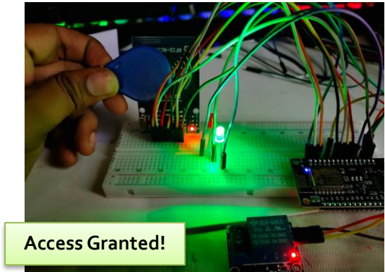
Fig 6: Card Authentication using RFID module
